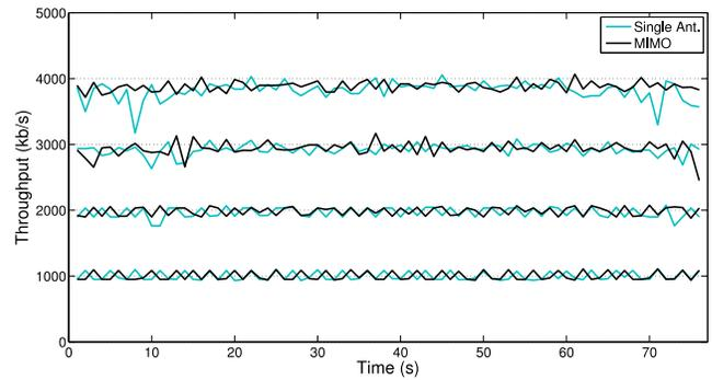
Fig. 4. UDP throughputs for various bitrate CBR traffic
