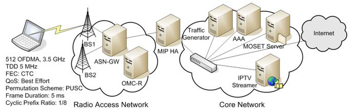
Fig. 1. Schematic of the Mobile WiMAX testbed
